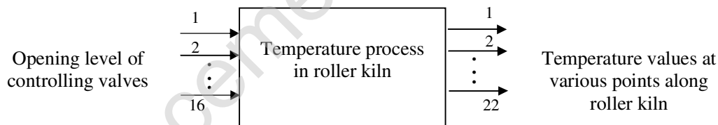
Fig. 7. Input and output variables of studied model.
