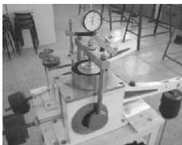
Fig. 4 Pressure-sinkage test apparatus of coal-bed
