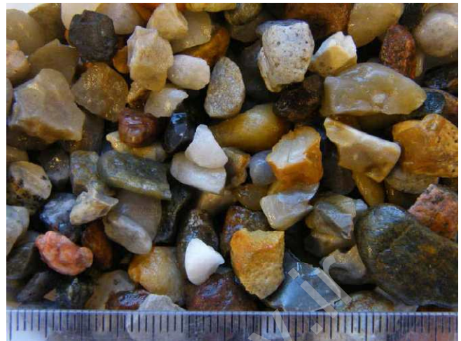
Fig. 8. -8+5 mm quartz particles as received. Each increment on the ruler represents 1 mm.
