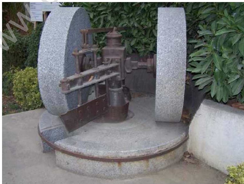
Fig. 1. The ancient oil mill is the ancestor of the modern VRM. The roller set is turned while the table is at rest.
