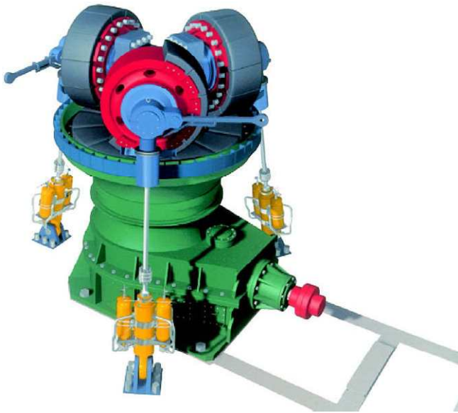
Fig. 2. The core components of the FLSmidth ATOX VRM. The horizontal circular table is driven by an electrical motor. Raw materials are added on the table. The raw materials are drawn underneath the rollers during operation. The frictional force between the table-bed-roller assembly ensures that the rollers will turn without any external power supply.
