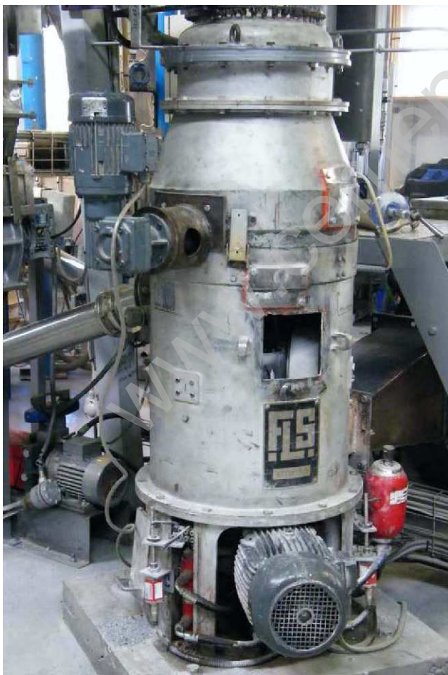
Fig. 6. FLSmidth ATOX laboratory VRM. The VRM has a height of approx. 1.5 m and is equipped with a static separator. The grinding force is generated by a hydraulic system and the table driven by an electric motor.
